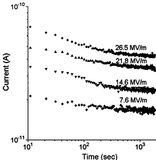
FIG. 2. Conduction currents at 100 °C as a function of time at various electric fields.
