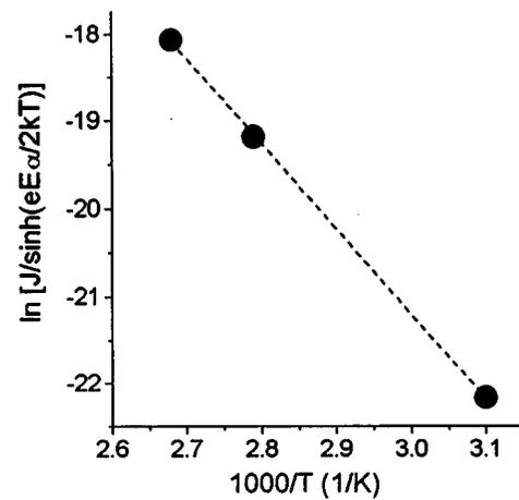
FIG. 6. Temperature dependence of current densities in PEI.
